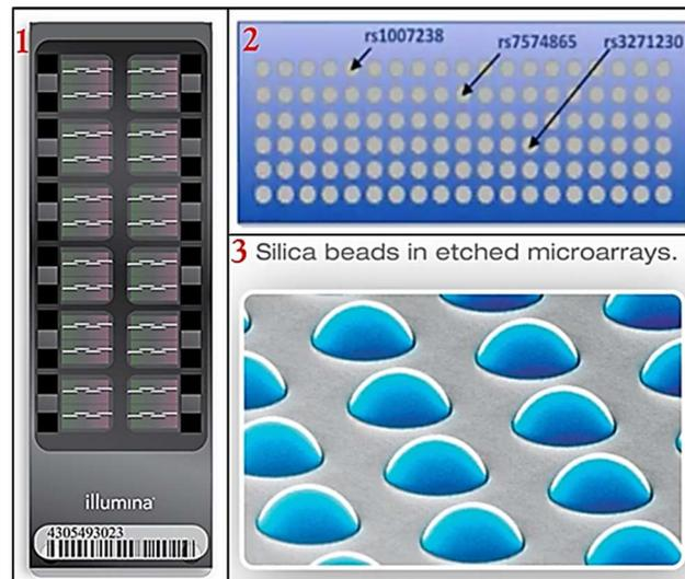
**Figure 2. Microarray Beadchip**
