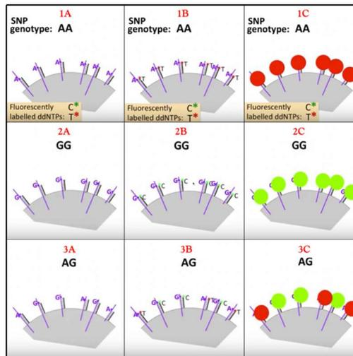
**Figure 5. Fluorescence Labeling to Determine Allele Values**
